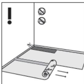
Important: installation with foil to the bottom
