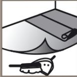
Clean and smoothen the subfloor, remove any grease; install the dampscreen and the subfloor; check the laminate planks for any damage.
