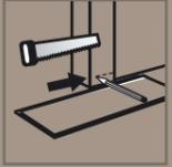
To measure **the height of the doorframe**, place a laminate plank against the doorframe, with the décor side down; mark the height and saw off the door and doorframe to the height marked. The laminate plank can then easily be pushed underneath the doorframe.
