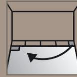
Take the cut-off part of the final plank in the previous row and use it to start the next row. Begin at the same side where you began the previous row and once again make sure that there is an 8 to 10 mm expansion joint between the laminate plank and the wall.
