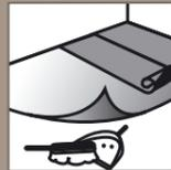
Once the floor has been cleaned and smoothed, the dampscreen and the subfloor installed, the laminate can be put in. Apply the dampscreen as follows: Lay out the dampscreen in long stretches over the entire floor.
