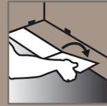
Roll the short side of the next laminate plank into the previous plank and press down against the groove of the previous row.
