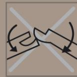
**To avoid damage to the connecting system it is strongly recommended never to roll a complete row in order to join it to the previous row.** Always make sure there is an 8 to 10 mm expansion joint between the laminate planks and walls or fixed objects.
