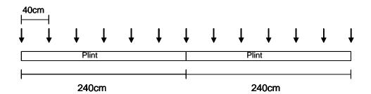
Note: it is recommended to use more clips with uneven walls. If the unevenness is too great, gaps between wall and skirting board are unavoidable.
