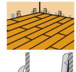
Important! Using Quick-Step® Clips has an impact on sawing mitres. The clips make the skirting board more of an angle. Use the tool supplied to saw perfect mitres for your skirting boards (see diagram).
